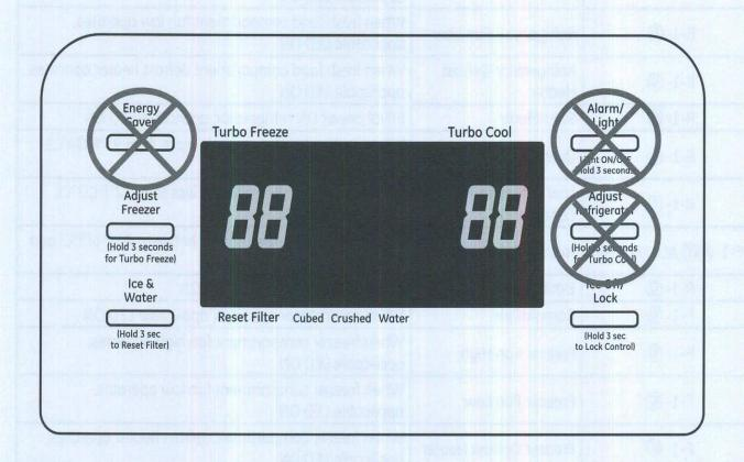
Segments of the figure "8"s will blink on and off corresponding to the loads that the main board has energized.
