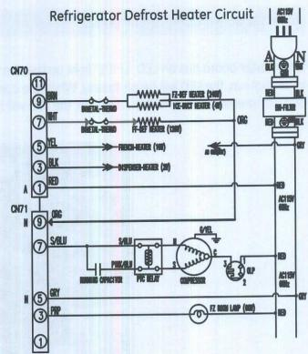
**Note:** To functionally test the defrost heaters, energize the heaters by using the test mode. (See *Test Mode Operation*.)
