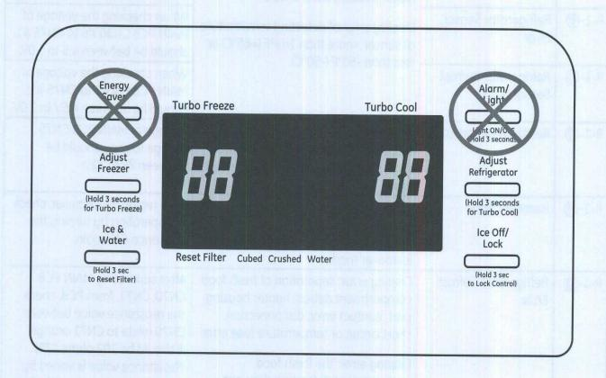
The self diagnostics mode will be displayed for 30 seconds, then the panel will return to normal display.
