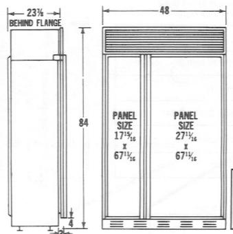
One 115 volt, 60 cycle, single phase 15 amp. A.C. wall outlet must be provided.
