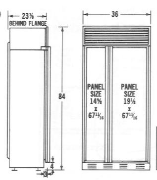
One 115 volt, 60 cycle, single phase 15 amp. A.C. wall outlet must be provided.
